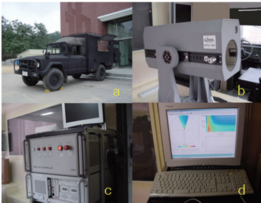
External view of MPSL a. Mobile system b. Lidar c. Control box & computer d. Display of measurement
