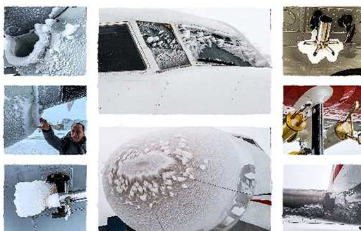
Ice accumulation on NRC Convair-580 after project flight sampling (Photo Credit: NCAR).
