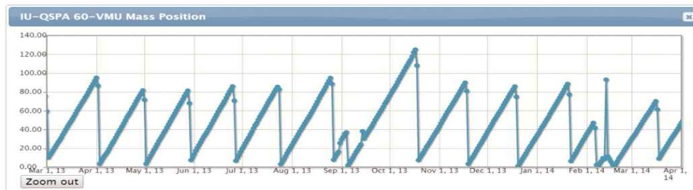
Fig. 7. Percentage of full-scale mass position output for the U module mass position of the STS-2.5 at IRIS/USGS (network code IU) station QSPA (Quiet South Pole, Antarctica) between March 1, 2013 and March 1, 2014. The slow gradual tilt in the ice causes the instrument's masses to go off center, requiring monthly re-centers of the instrument. The vertical axis defines the percentage of the operational mass position range and is specific to the sensor and defined in the metadata for the mass position channels.
