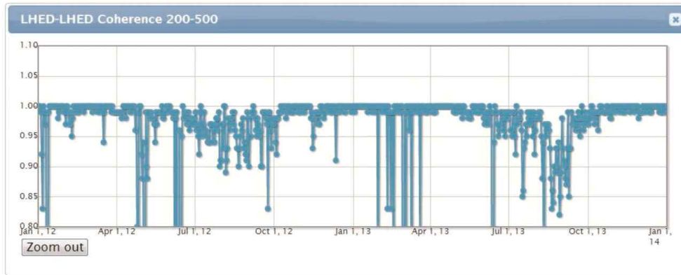
Fig. 14. Average magnitude-squared coherence from 200 to 500 s period between the derived East-West long period components of the STS-1 (location code 00) and STS-2.5 (location code 10) at IRIS/USGS (network code IU) station CCM (Cathedral Cave, Missouri, United States) between January 1, 2012 and December 31, 2013 (top). The
