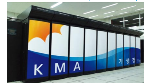
► KMA 3 rd Supercomputer Cray XE6 "Haeon"
